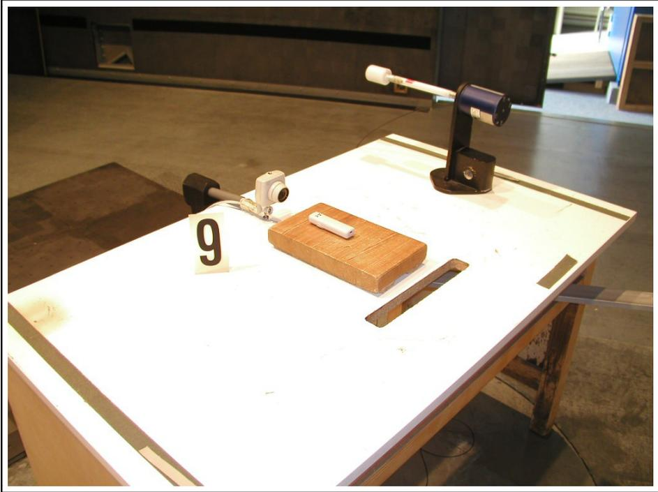
Figure 2 : Test Set-up "Radiated electromagnetic fields and immunity to radiated electromagnetic fields"
