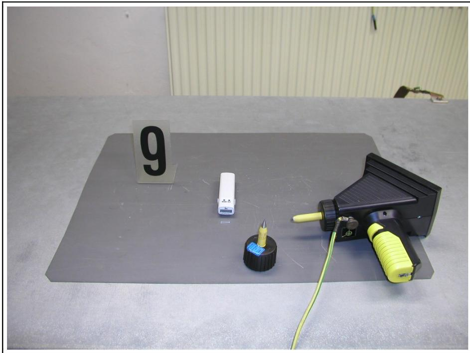
Figure 3 : Test Set-up "Immunity to electrostatic discharge (ESD)"
