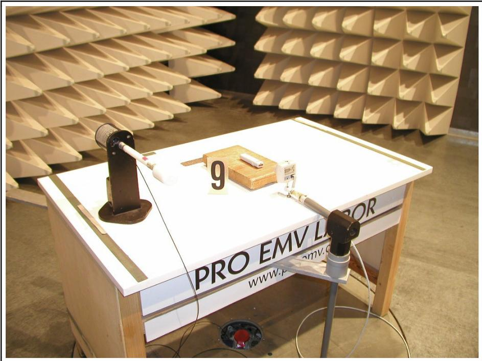
Figure 1 : Test Set-up "Radiated electromagnetic fields and immunity to radiated electromagnetic fields"
